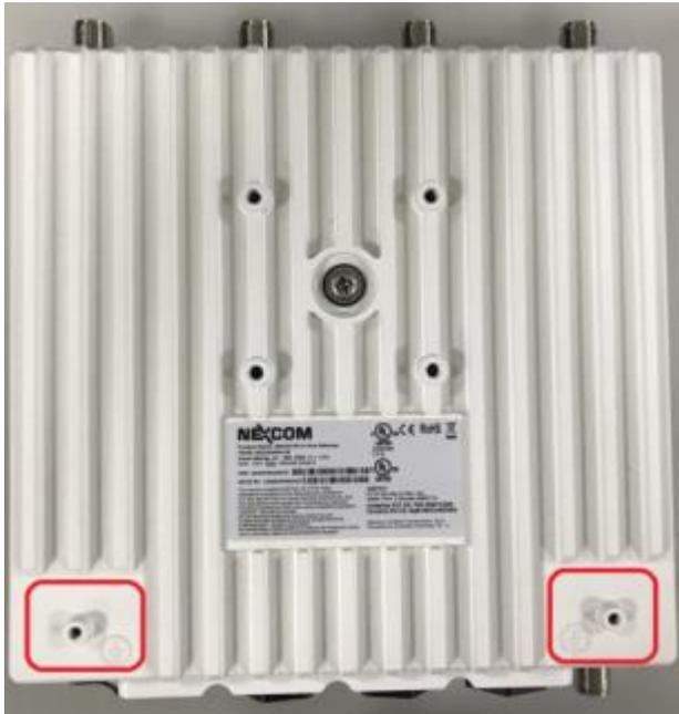
1. Be sure to ground the 0.75mm<sup>2</sup> ground screw with an appropriate grounding wire ( Earth, Green/Yellow wire 18AWG, not included) by attaching it to a good earth ground connection.
