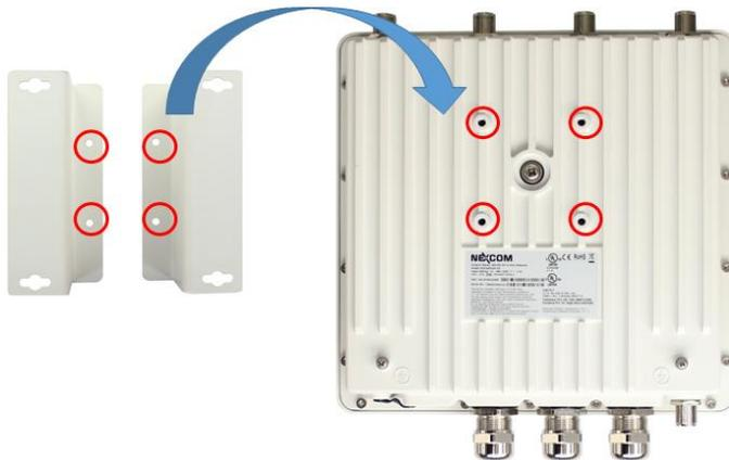
2. Be sure to fasten the mounting kit with horizontal position as below:
