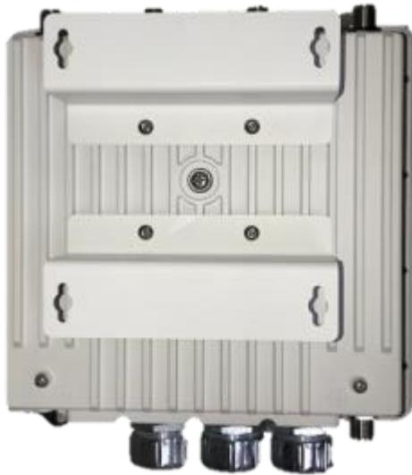
3. Hang on NIO200 to the wall with water proof connector at the bottom direction.
