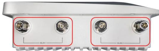
Wi-Fi antenna connector for Wi-Fi Mesh connection (WLAN 1 & WLAN 2)
